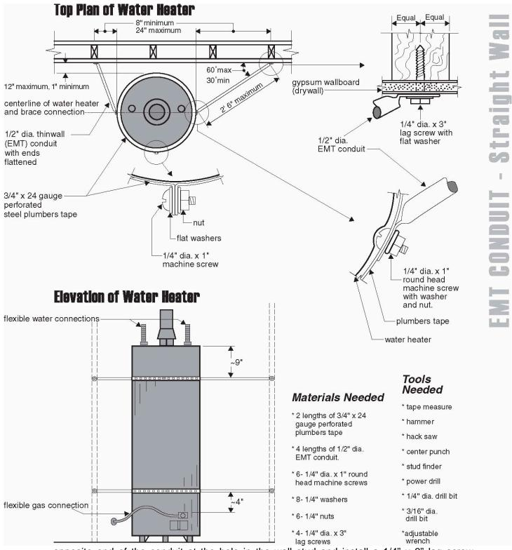
opposite end of the conduit at the hole in the wall stud and install a 1/4" x 3" lag screw. Repeat this procedure for the other three conduits.
