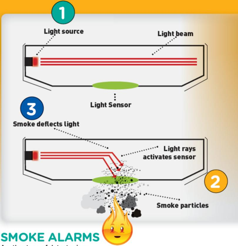
Another type of detector is an photoelectric smoke alarm. Here's how it works:
